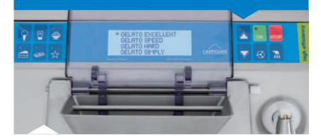
All commands remain accessible when the hopper cover is open so that the op-
